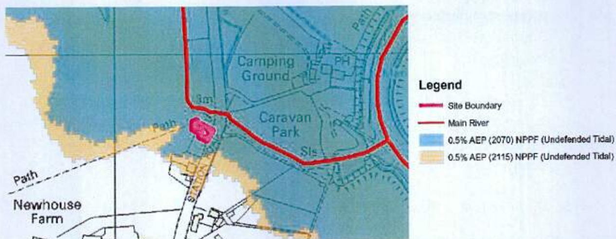
FIGURE 2.2.2.2 MODELLED FLOOD OUTLINE 0.5% AEP UNDEFENDED TIDAL
