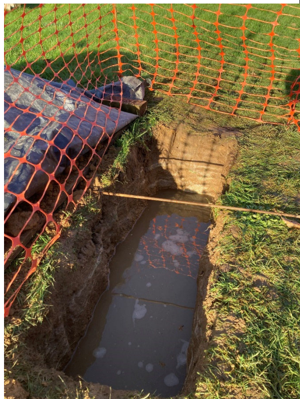
Photograph 4 : Trial Pit TP2 under test
