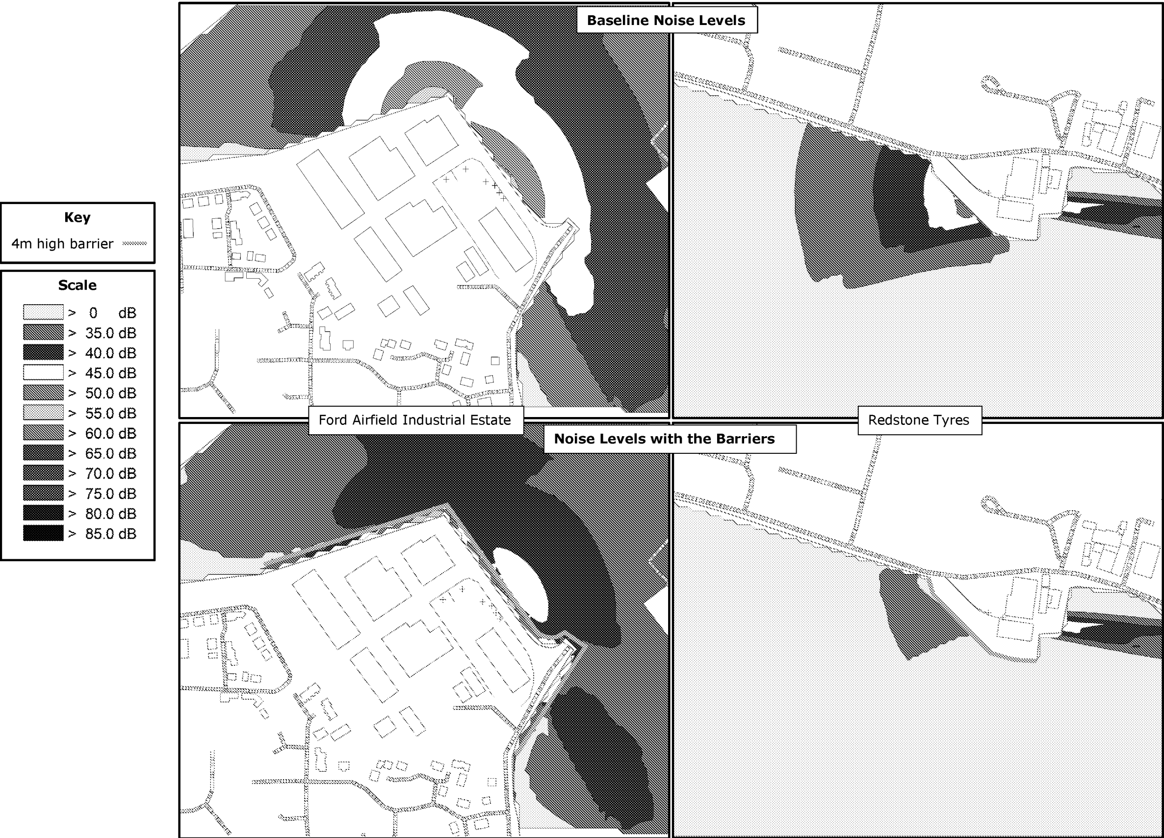
Figure 7: Noise Modelling of the Baseline Noise Levels (Top) and with the Noise Barriers (Bottom)
