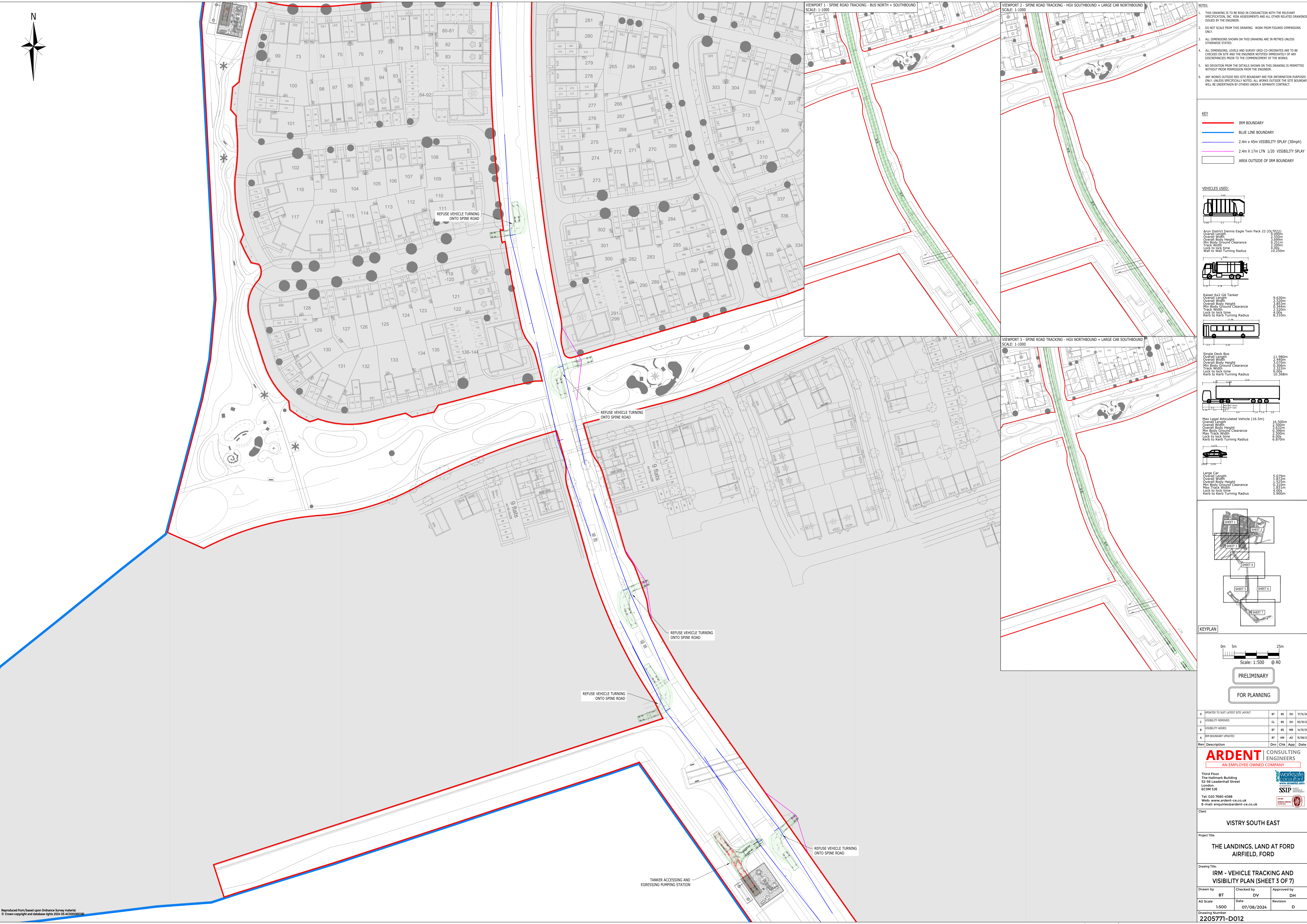
VIEWPORT 1 - SPINE ROAD TRACKING - BUS NORTH + SOUTHBOUND SCALE: 1:1000
