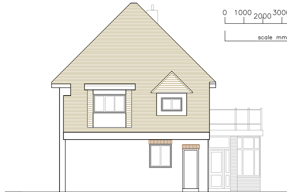
EXISTING WEST ELEVATION 1:100
