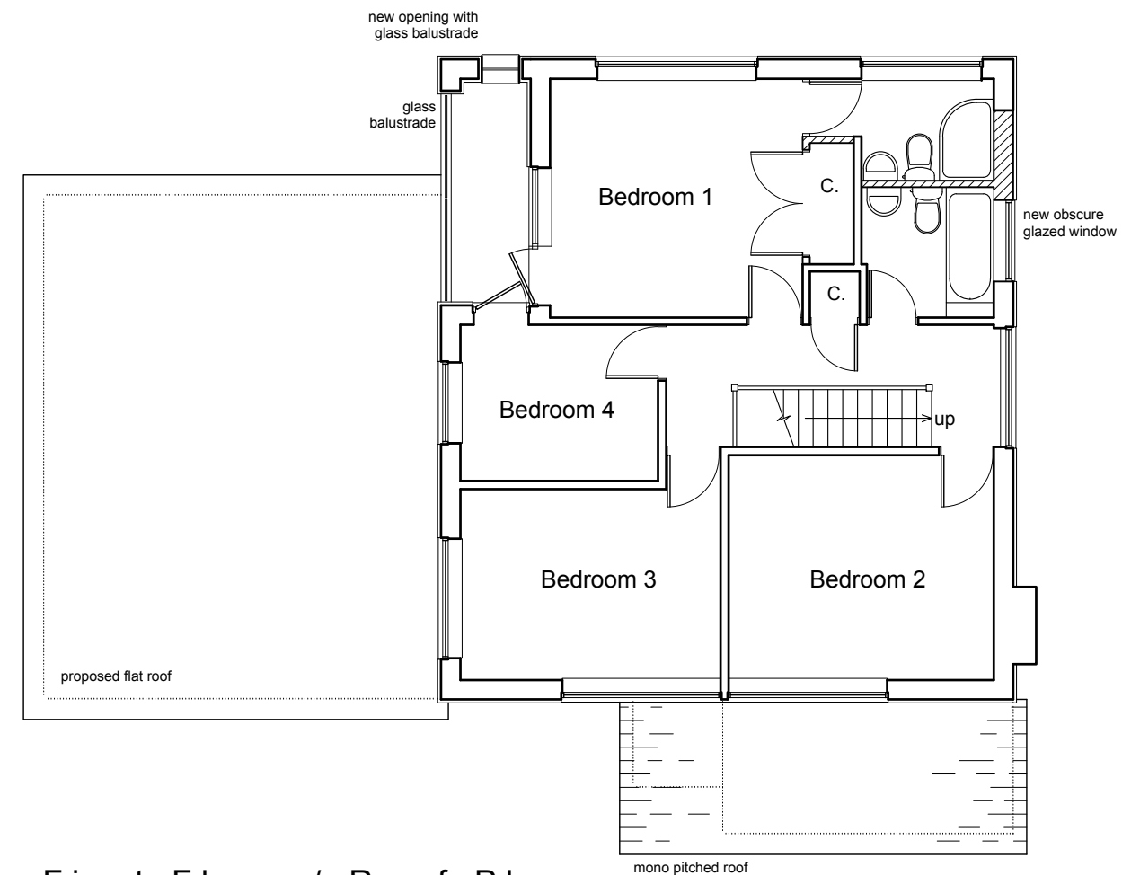
First Floor / Roof Plan
