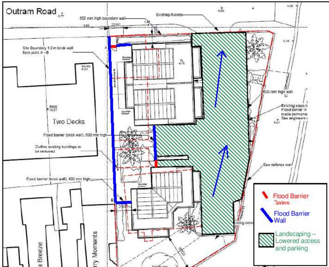
Figure 13 -Proposed flood proofing and landscaping
