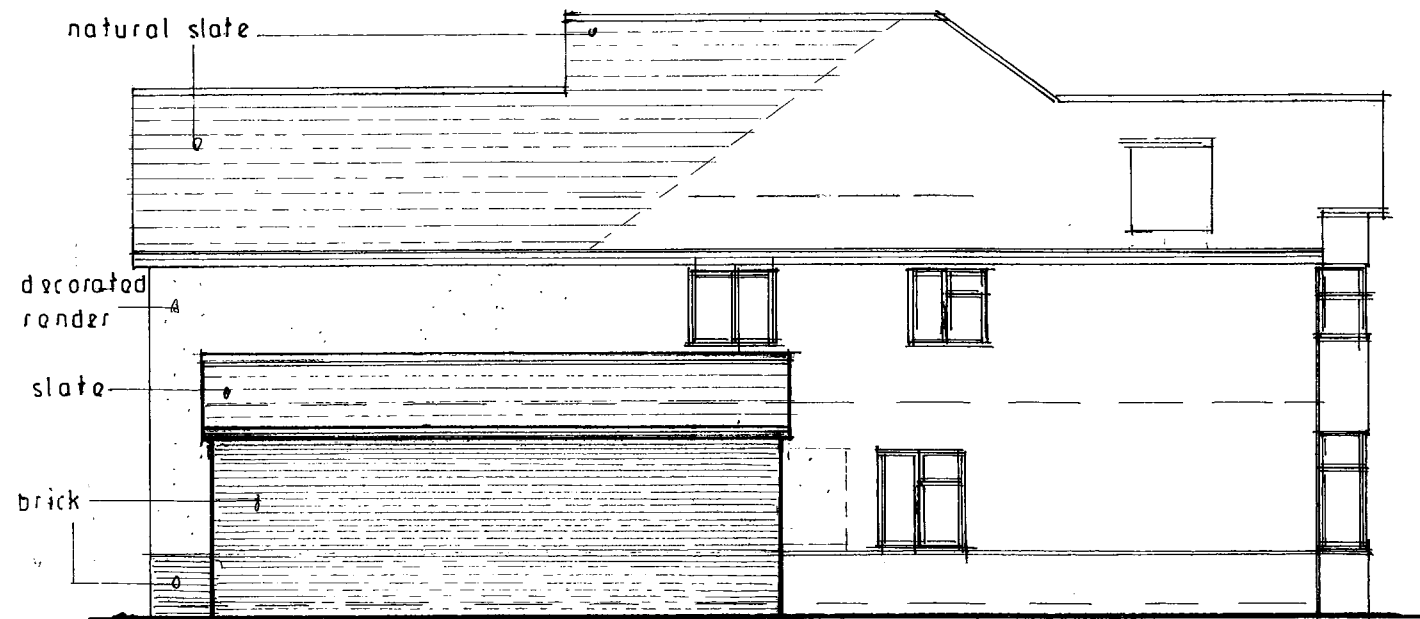
Proposed West Elevation
