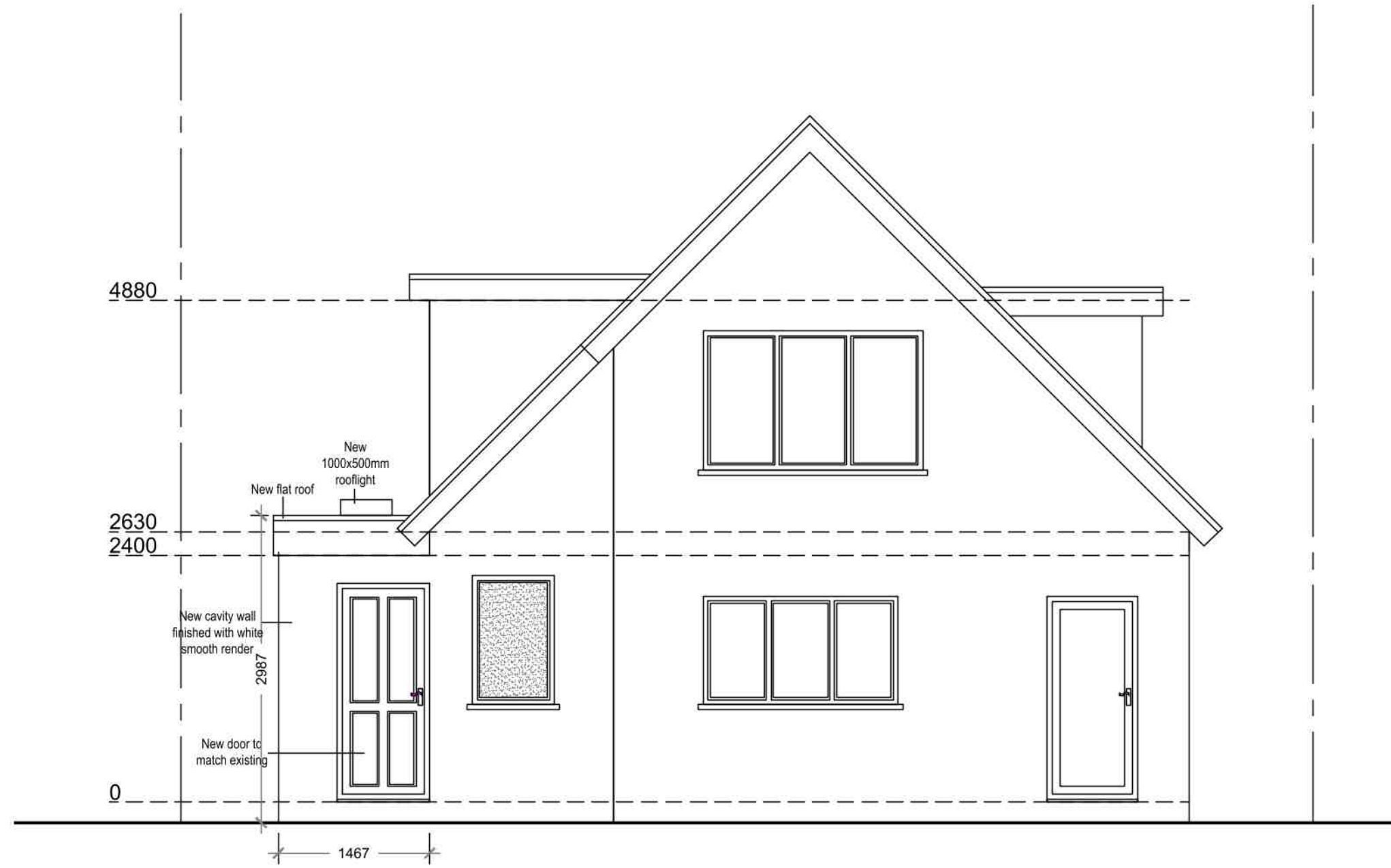
Proposed East Elevation Scale 1:50
