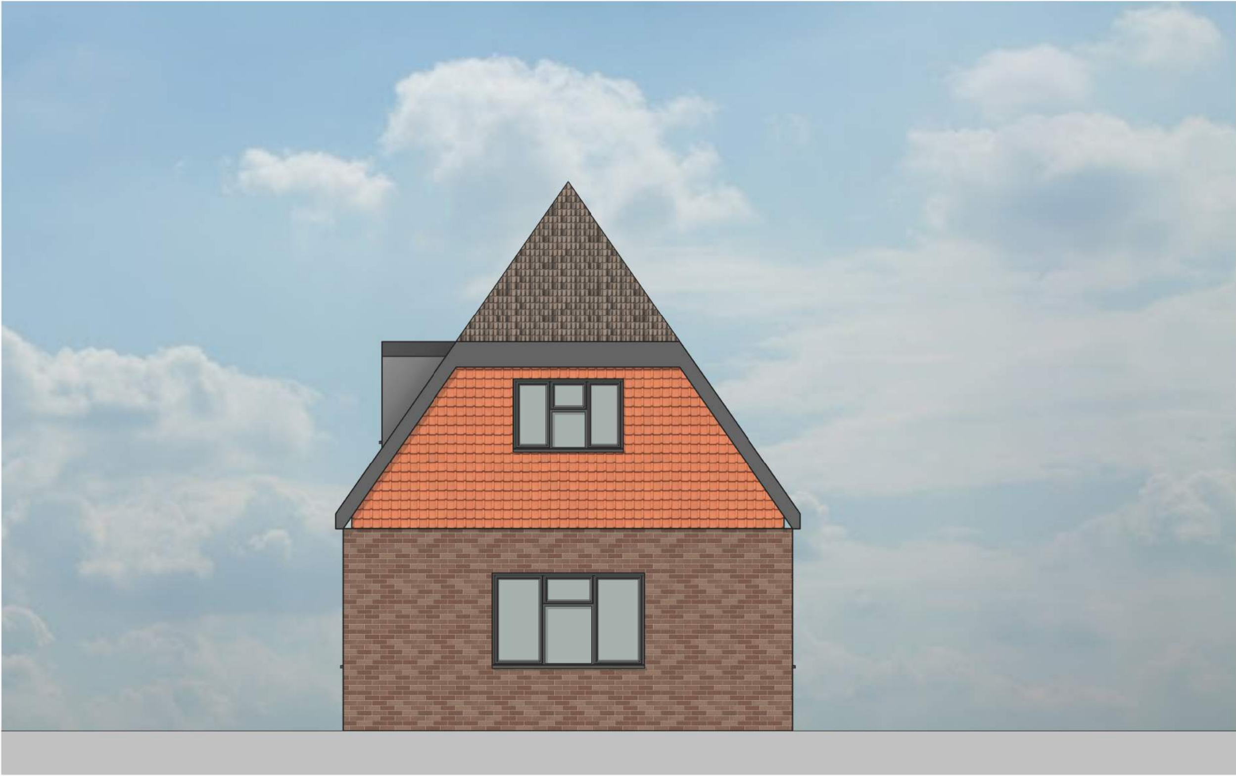
Existing North Elevation 1 : 50
