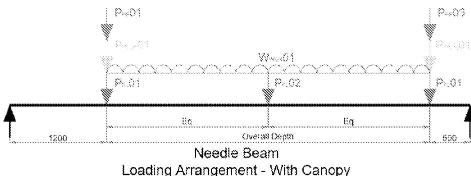
$P_{r,01} = W_{w,x} \times S_x \times (D / 2 + 0.7)$  - Point Load due to Roof & Canopy
