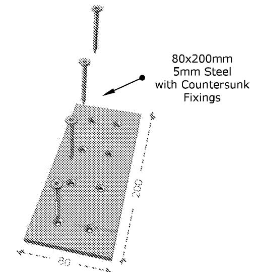
Floor Connection Plates to be set 400mm from Cassette Edge to Plate Centre
