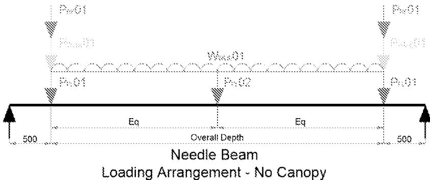
$P_{r,01} = W_{w,x} \times S_x \times D / 2$  - Point Load due to Roof
