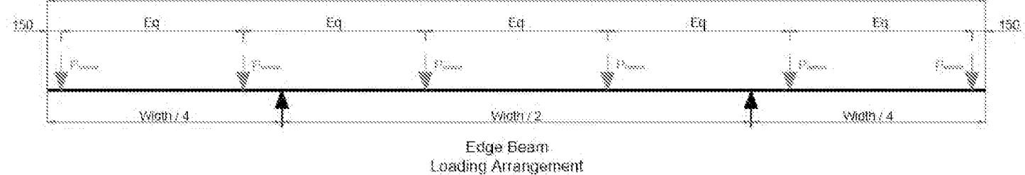
$P_{needle}$  to be taken as R-02 from the relevant Needle loading case. To reduce the number of cases assessed, the load from the Maximum width will be taken ie Load Cases A-05, B-05, C-05, A-10, B-10 & C10. Edge beams will be assessed for cases with Max Cassette widths of 1.9m & 2.3m
