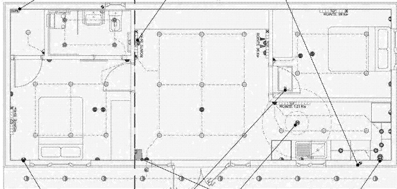
All Internal Power Sockets & Light Switches to be Located Between 450mm Min. to 1300mm Maximum to comply with Part M Building Regulations, Unless the Annex is specifically designed for a person with Limited Reach
