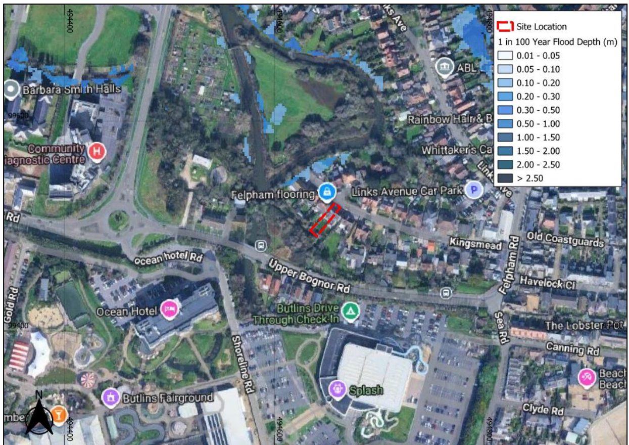
Figure 8: 1 in 100 Year Depth (Base map and data from Google Hybrid © Contains public sector information licensed under the Open Government Licence v3.0)
