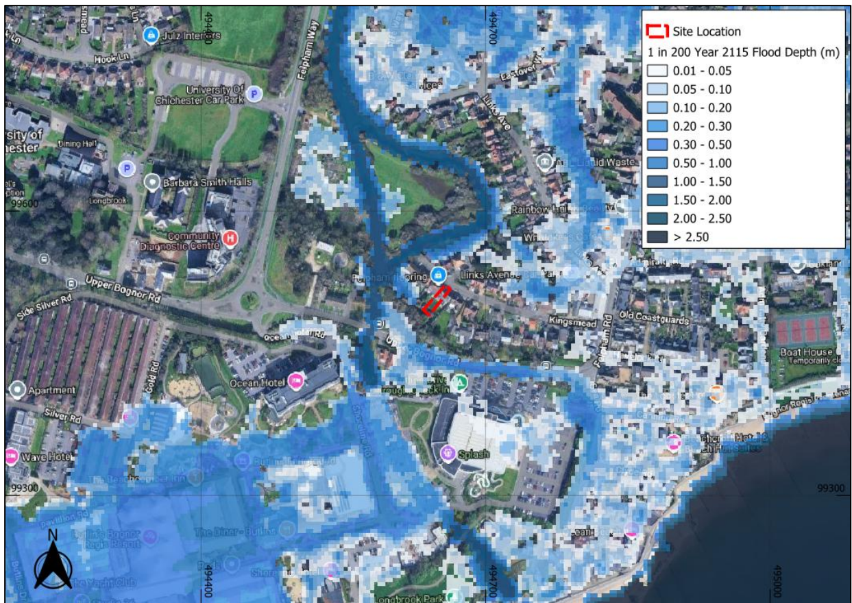
Figure 12: 1 in 200 Year 2115 Flood Depths (Base map and data from Google Hybrid © Contains public sector information licensed under the Open Government Licence v3.0)
