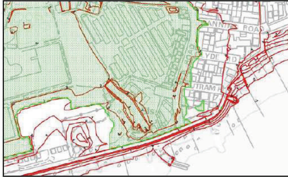
Figure 12 - 1 in 200yr tidal breach event floodplain
