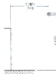
Measuring location (discharge side)
