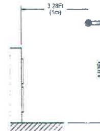
Measuring location (discharge side)
