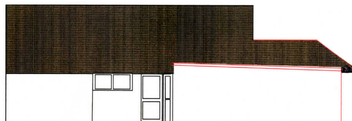
North elevation (facing 13 Ashmere lane) proposed
