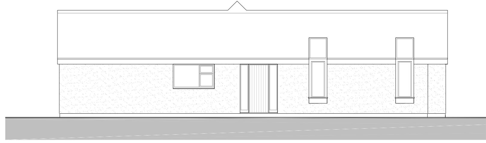
PROPOSED SIDE ELEVATION showing slot windows integrated with Velux
