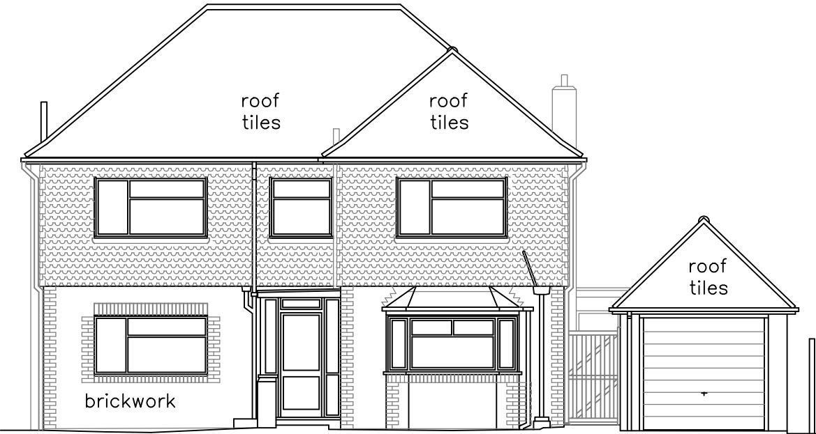
South Elevation (Front)
