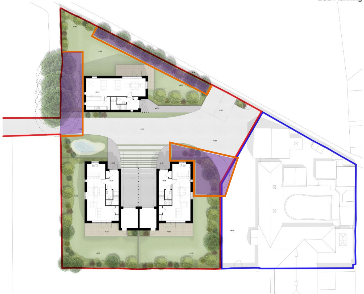
Figure 3- Extent of Tree Protection Measures
