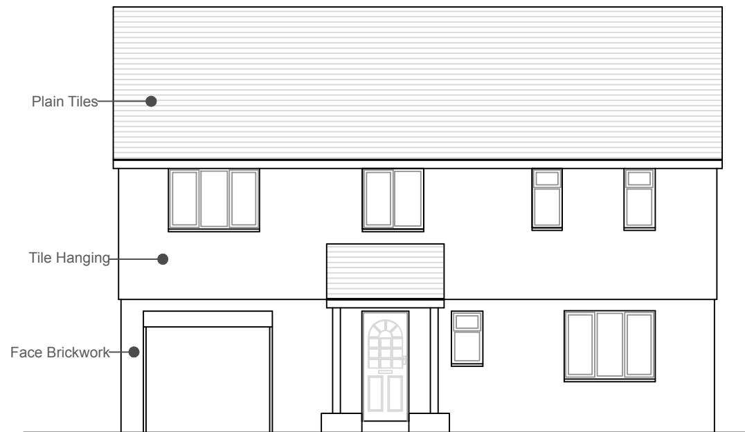
Front Elevation (north)
