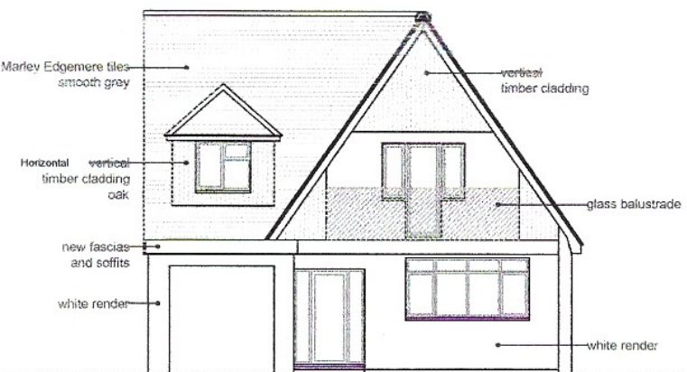
Front Elevation (west)
