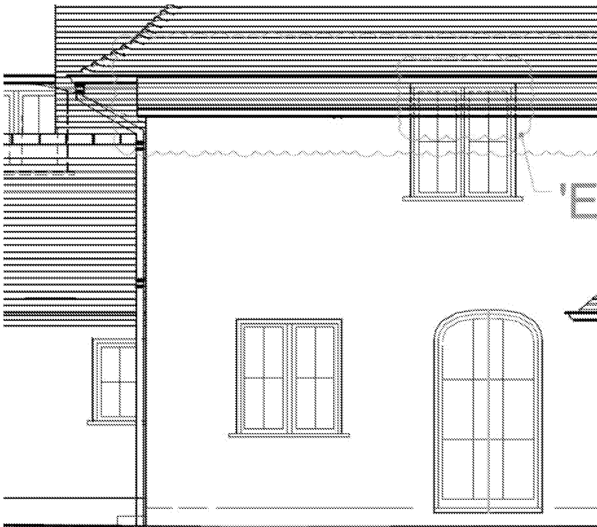
Figure 2 - Proposed Western Elevation showing rain water guttering
