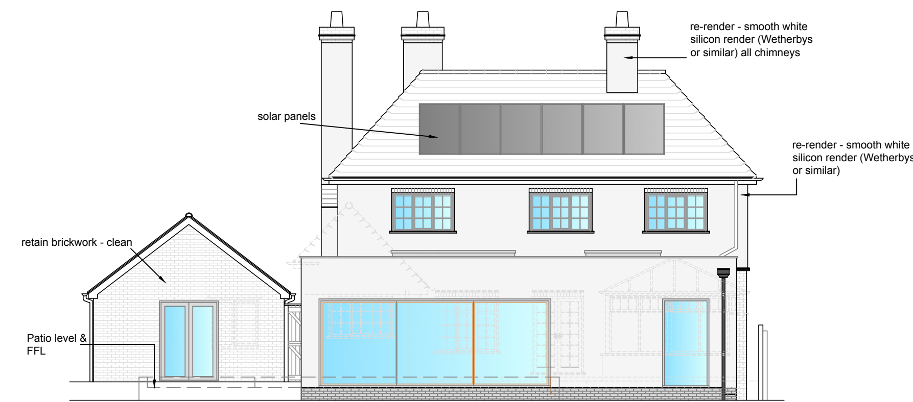
South Elevation (Rear)
