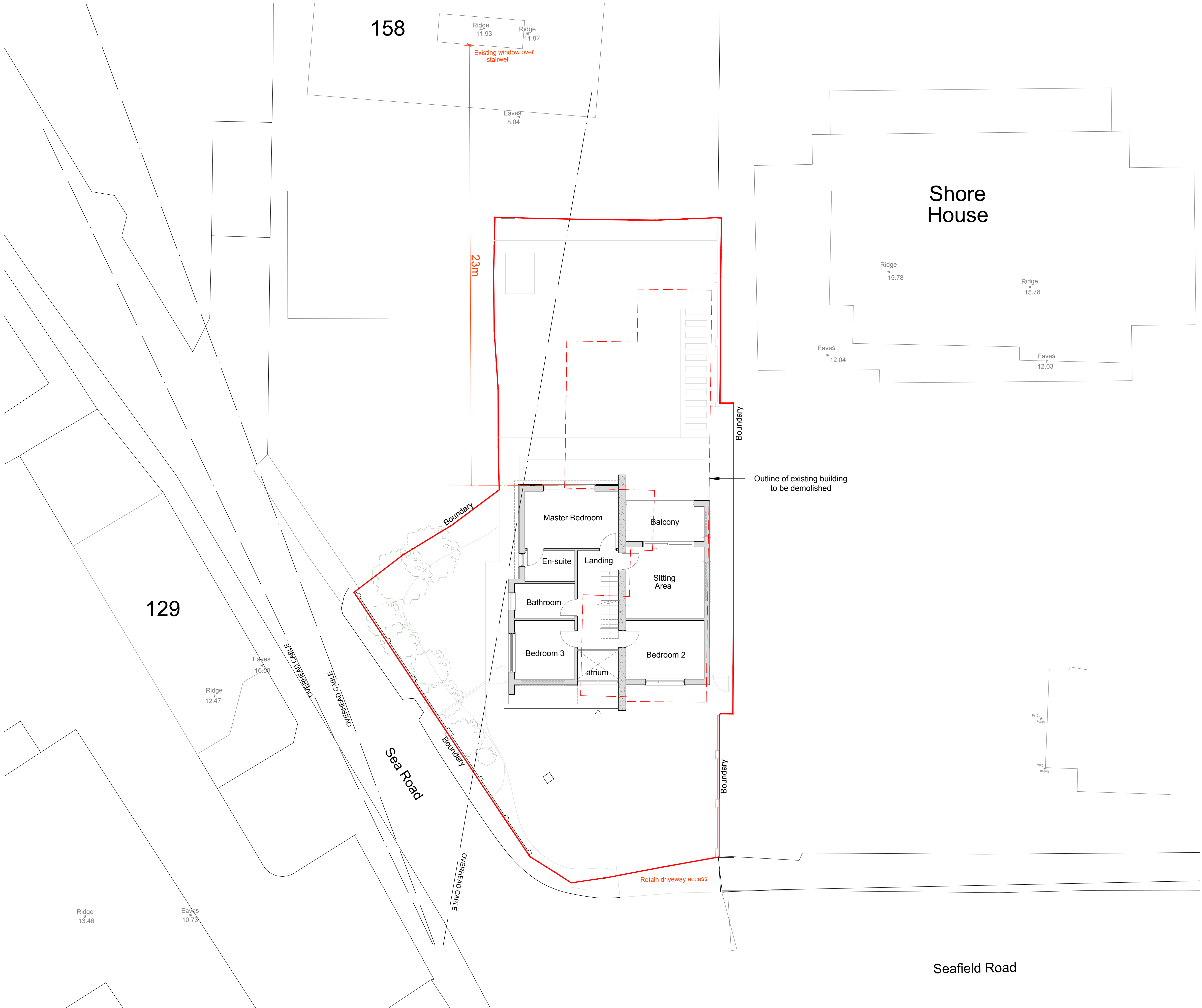
First Floor Plan with context 1:100
