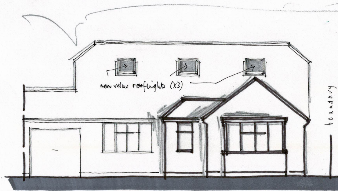
FRONT (s) ELEVATION 1:100 @ A3 0 1 2 3 4 5m metres
