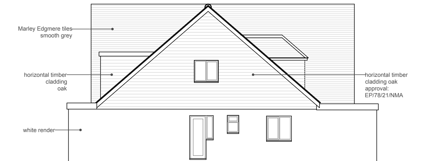
Side Elevation (north)
