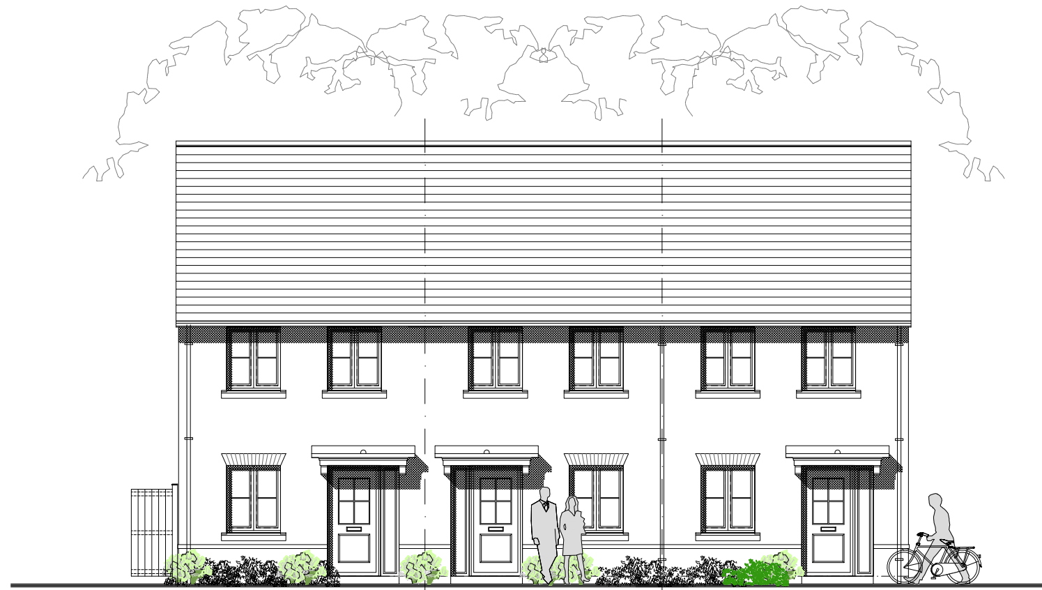
Plot 27 202L Plot 26 202L Plot 25 202L FRONT ELEVATION Note : Wall areas left clear to elevations are in facing brickwork
