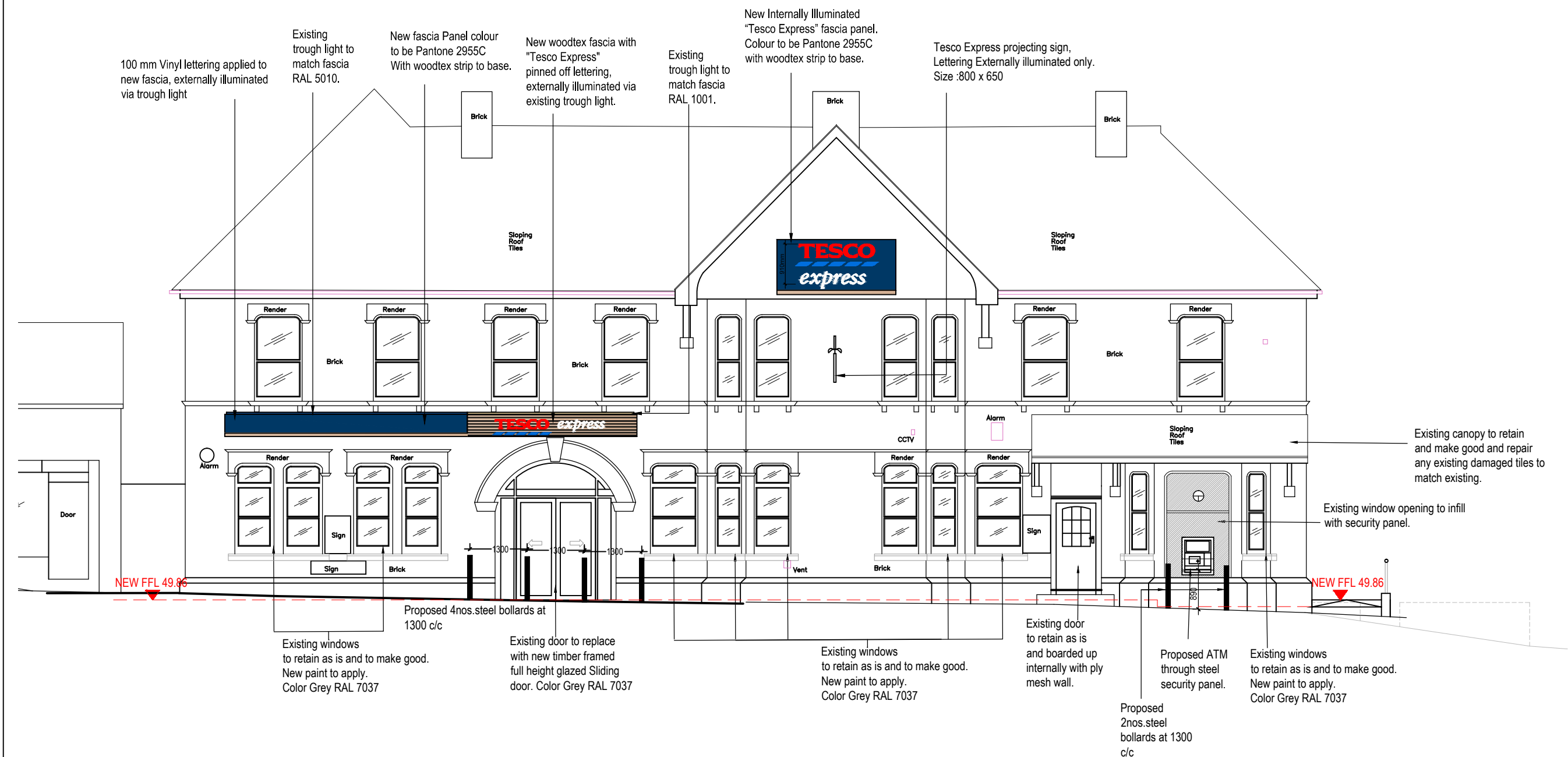
FRONT ELEVATION-A AS PROPOSED SCALE 1:100
