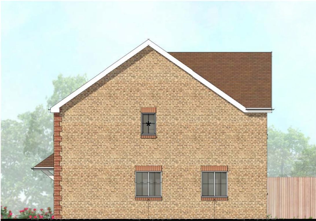
Side Elevation B 1 : 100 high level window (< 1sqm opening) 1200mm height on plot 238 ONLY window to plot 238 ONLY
