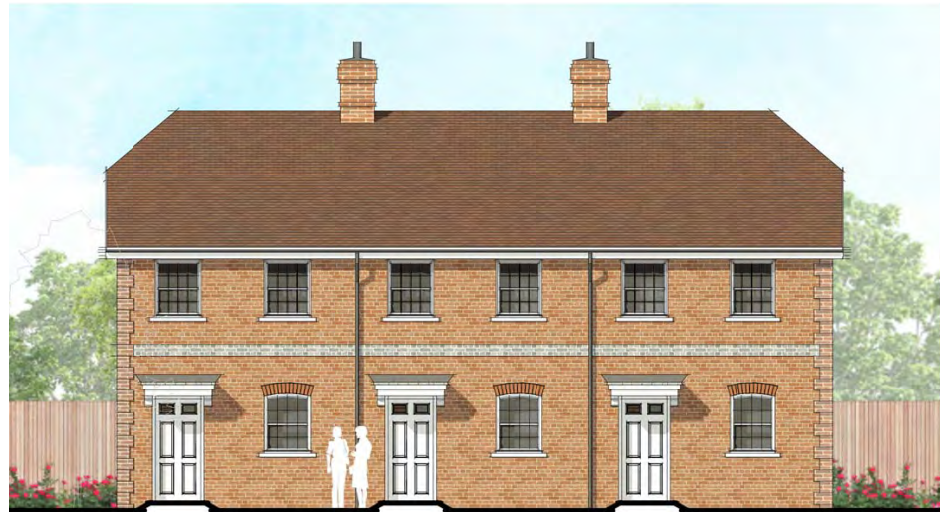
Block B - Terrace Orange English Bond brick with grey banding to match The Well House
