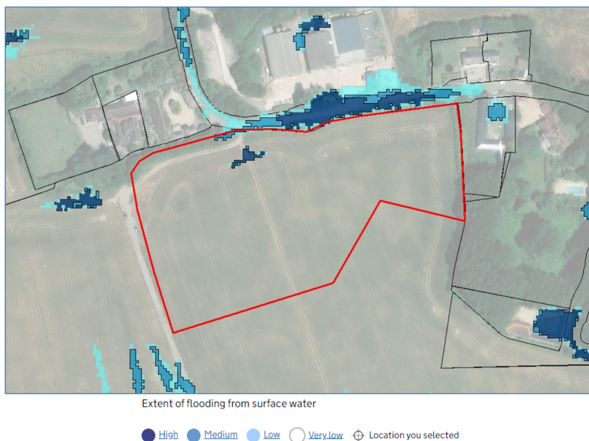
Figure 3 - extract from the EA's Long-Term Risk of Flooding from Surface Water (RoFSW) maps for the yearly chance of flooding between 2040 and 2060
