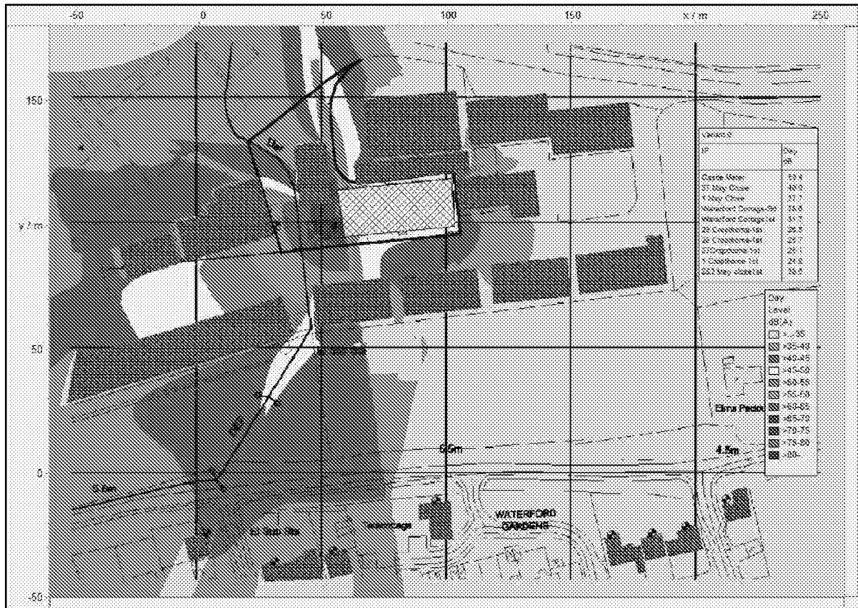
Figure 20. Current Sound Propagation (82dB L_{Aeq,1minute} ) 18:00-21:00 hours
