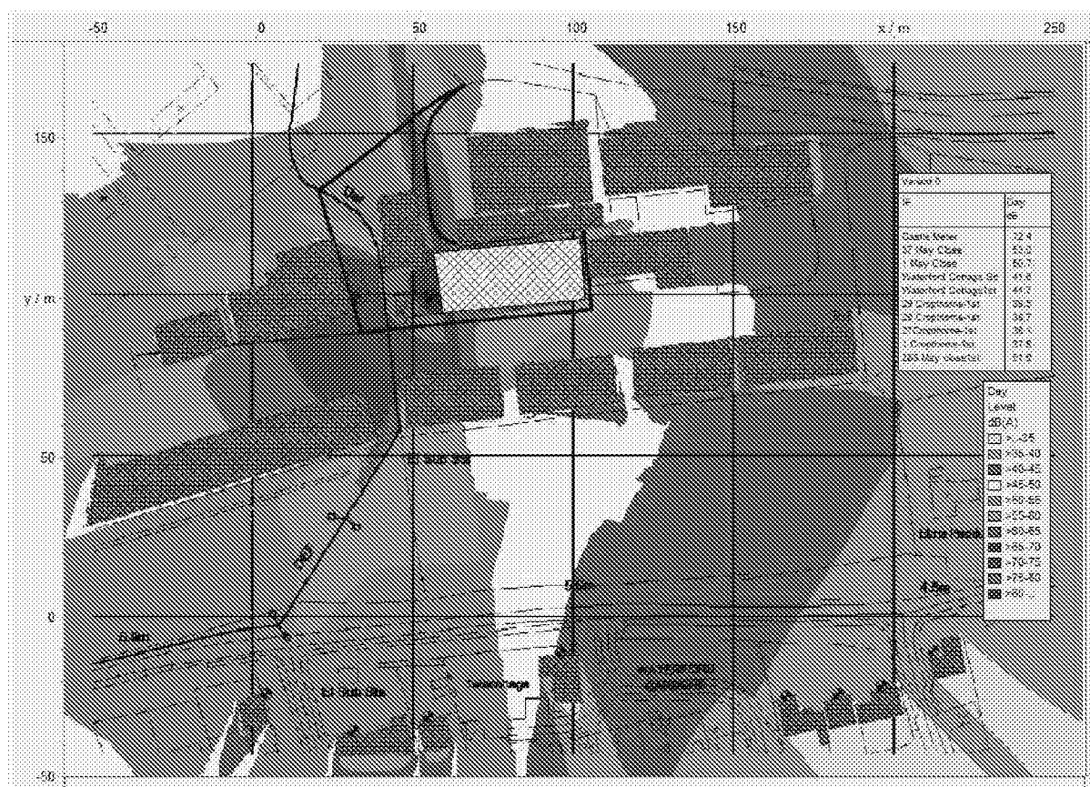
Figure 22. Sound Propagation using 95dB L_{A_{Max}} inside the factory premises
