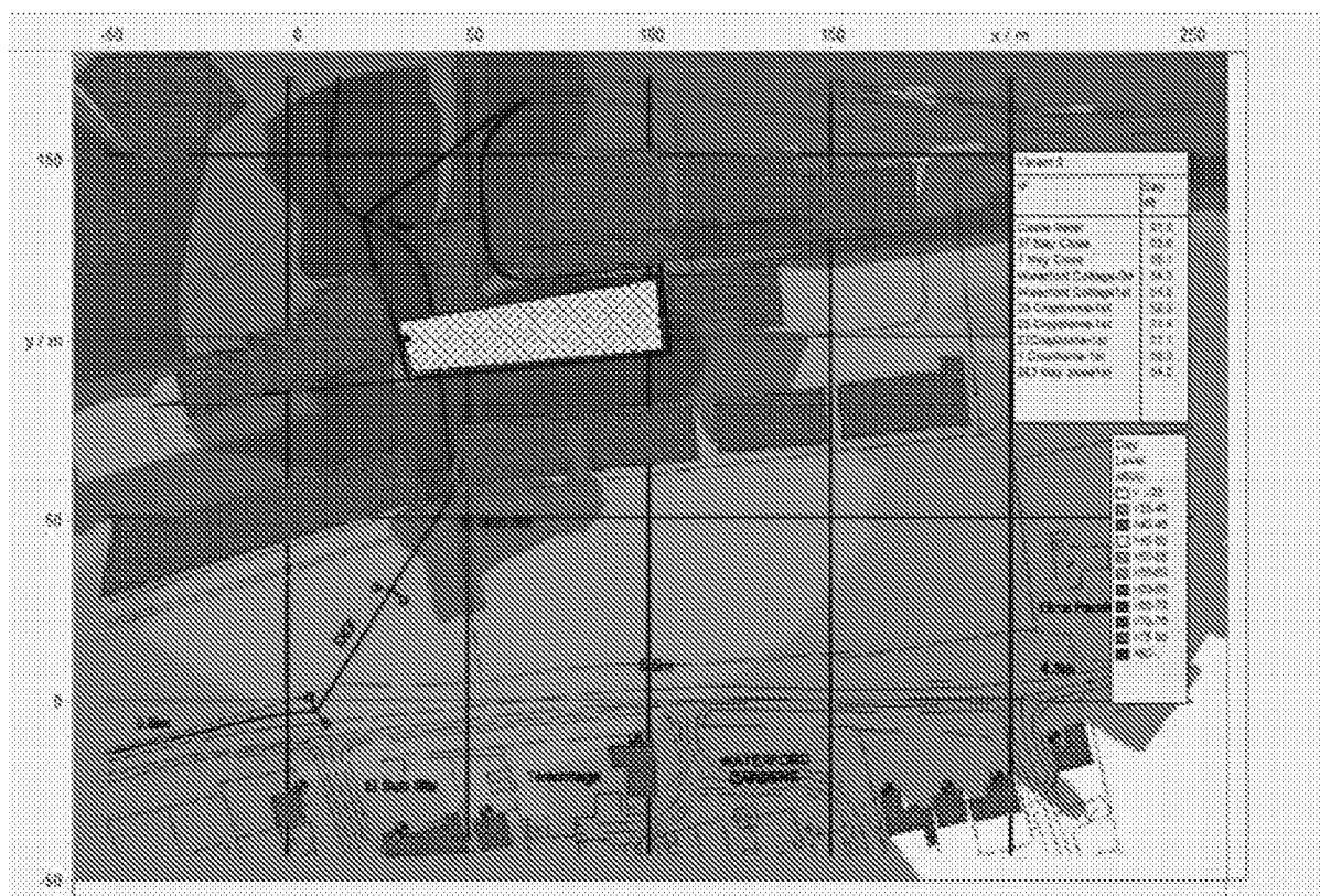
Figure 25. Partially Enclosed Yard using 113 dB L_{Amax}
