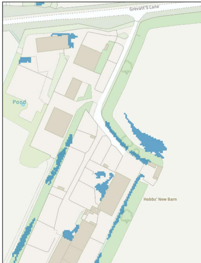
Figure 2.2 Surface Water Flood Risk (1 in 100yrs) Source: Environment Agency
