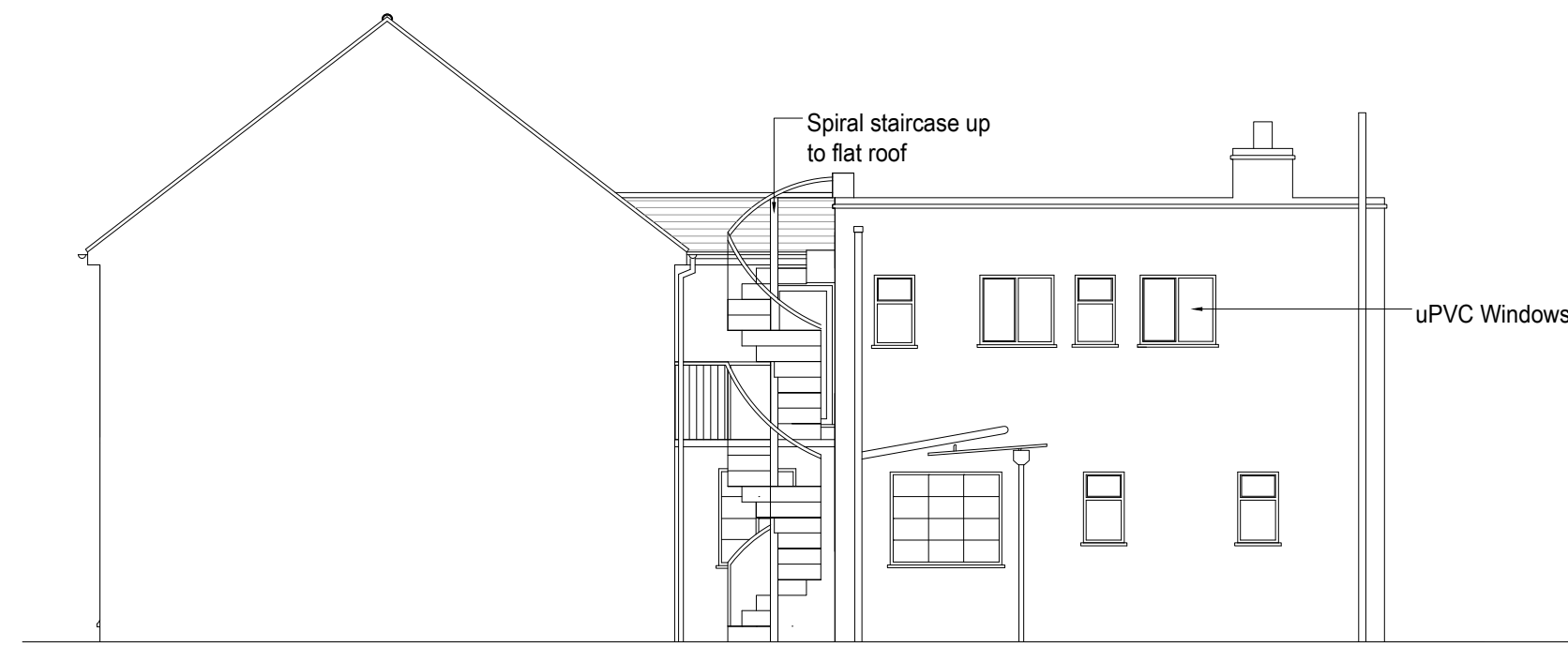
Existing Side (West) Sectional Elevation 1:100
