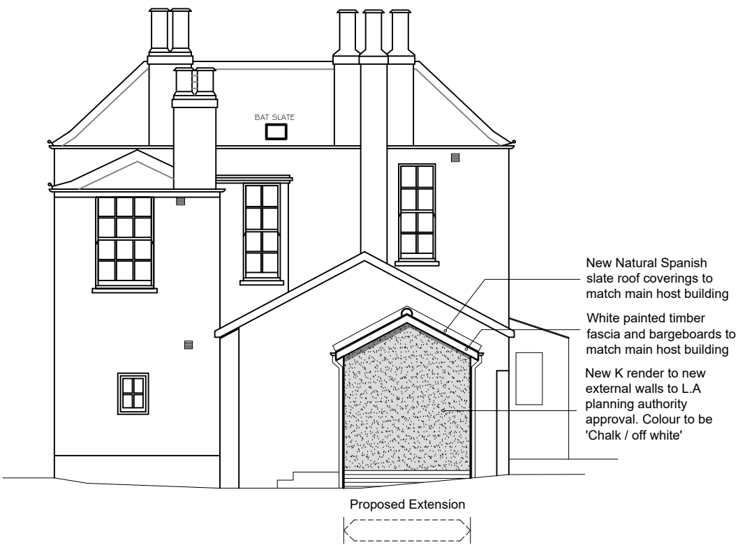
PROPOSED EAST ELEVATION
