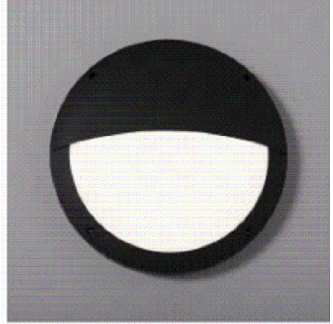
New Emergency lighting with microwave sensor 16-18W, 3000K IP44 Rating 1.6m from FGL
