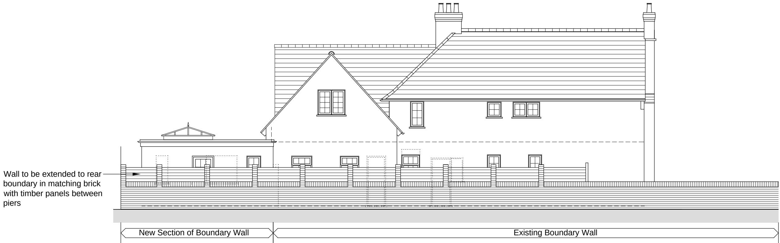
PROPOSED NORTH EAST ELEVATION (SHOWING BOUNDARY WALL) @ 1:100@ 1:100
