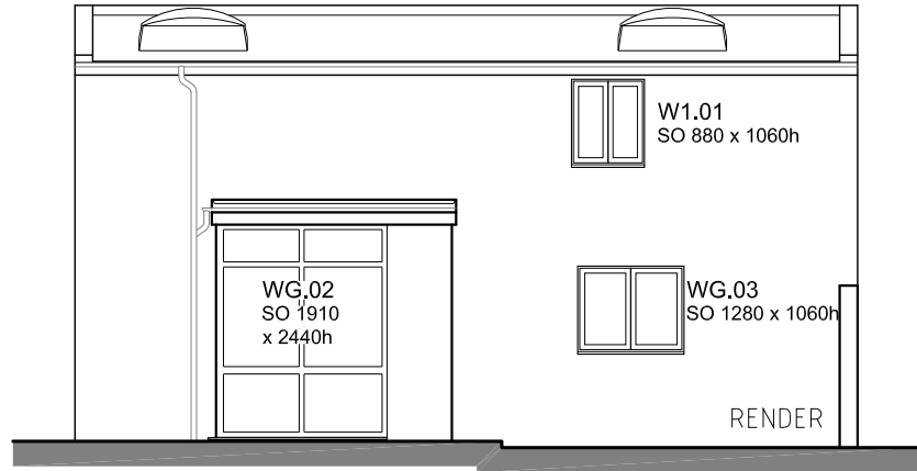
EXISTING NORTH FACING ELEVATION Sc. 1:100
