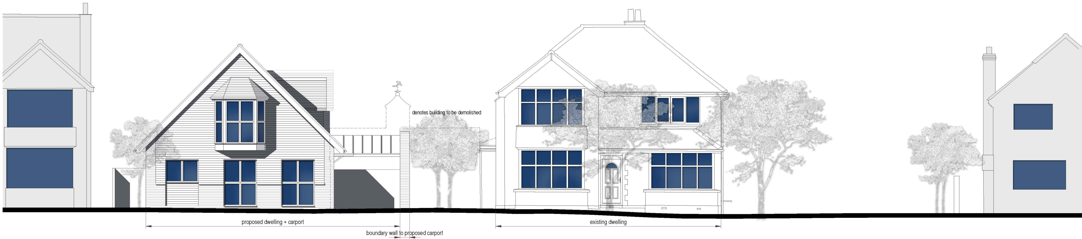
SOUTH ELEVATION - MATERIALS - Roof - Plain Tiles / Walls - Face Brickwork + Tile Hanging / Windows - White PVC-u , Front Door - Dark Green PVC-u, Folding Doors - Anthracite Grey - RAL7016 / RW Goods - PVC-u / Carport Roof - Standing Seam
