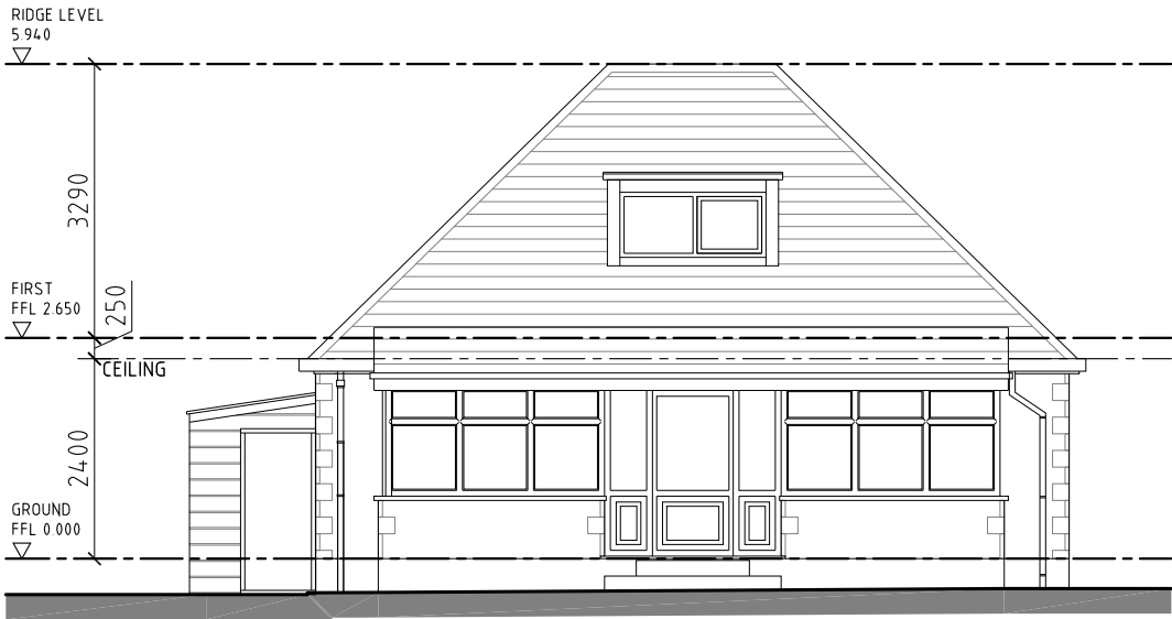
EXISTING NORTH FACING ELEVATION Sc. 1:100
