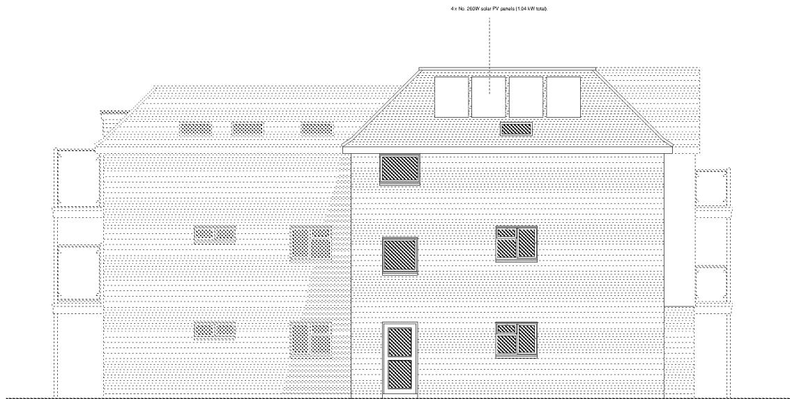
Figure - South-West elevation showing solar PV panels on the roof.
