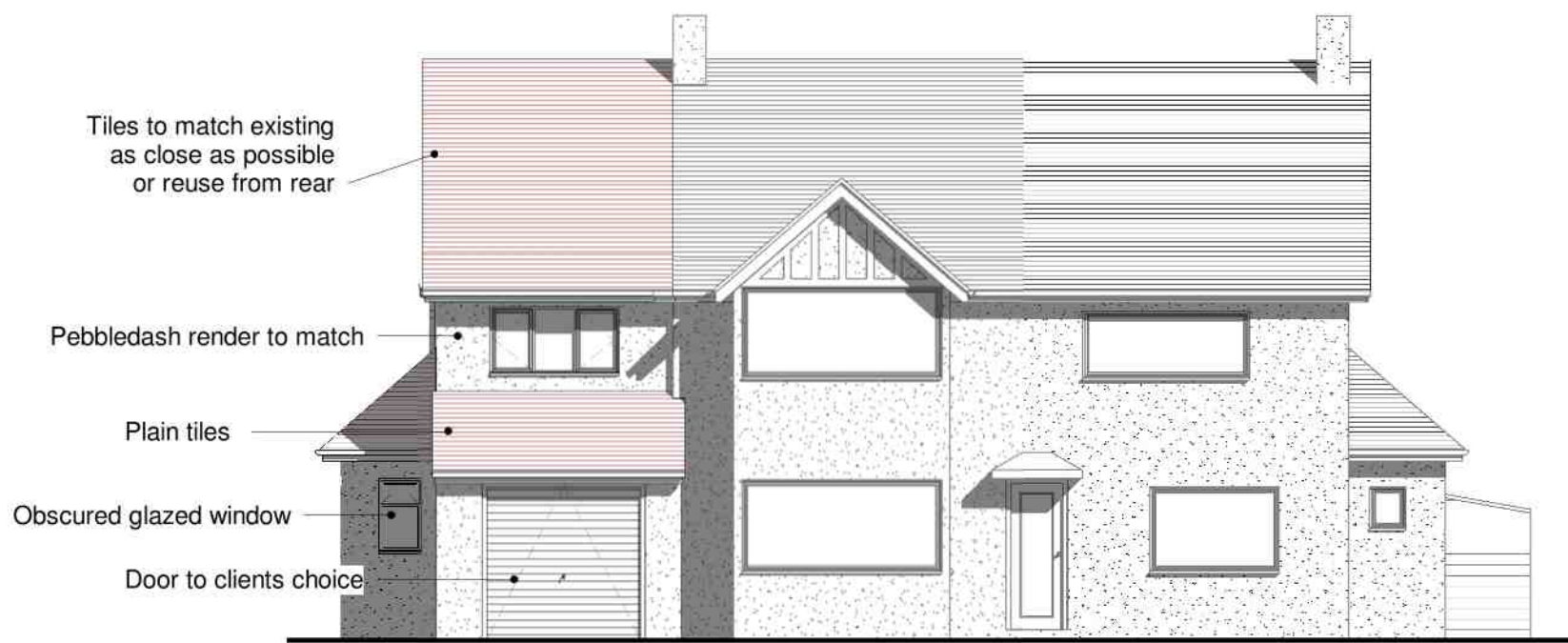
2 East (Front) Elevation Proposed 1 : 100
