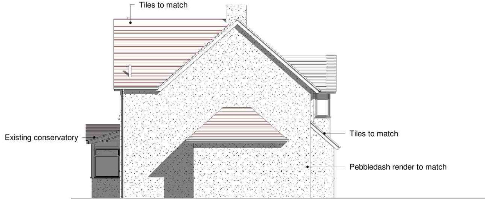
6 South (Side) Elevation Proposed 1 : 100
