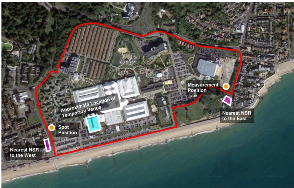
Figure 1: A site plan showing the site boundary of the Butlin's site in red, as well as the locations of the measurement positions, nearest noise sensitive receiver and the approximate location of the proposed venue. Imagery courtesy of Google.
