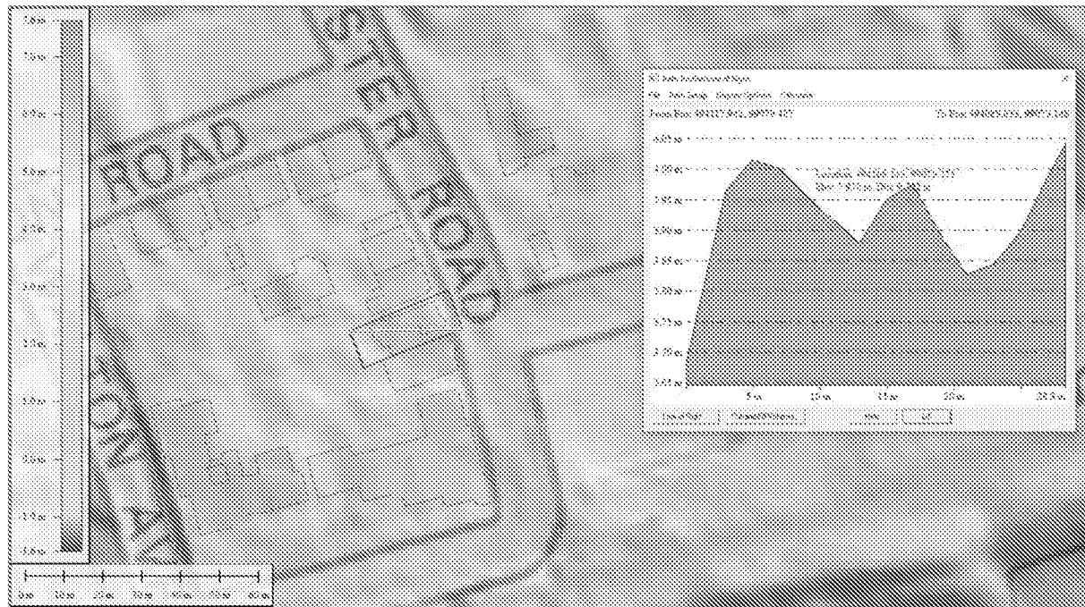
Figure 3: 2m resolution LiDAR DTM showing topographic levels across the site (transects runs from southeast to northwest) (Source: EA LiDAR, OS Mapping overlain)
