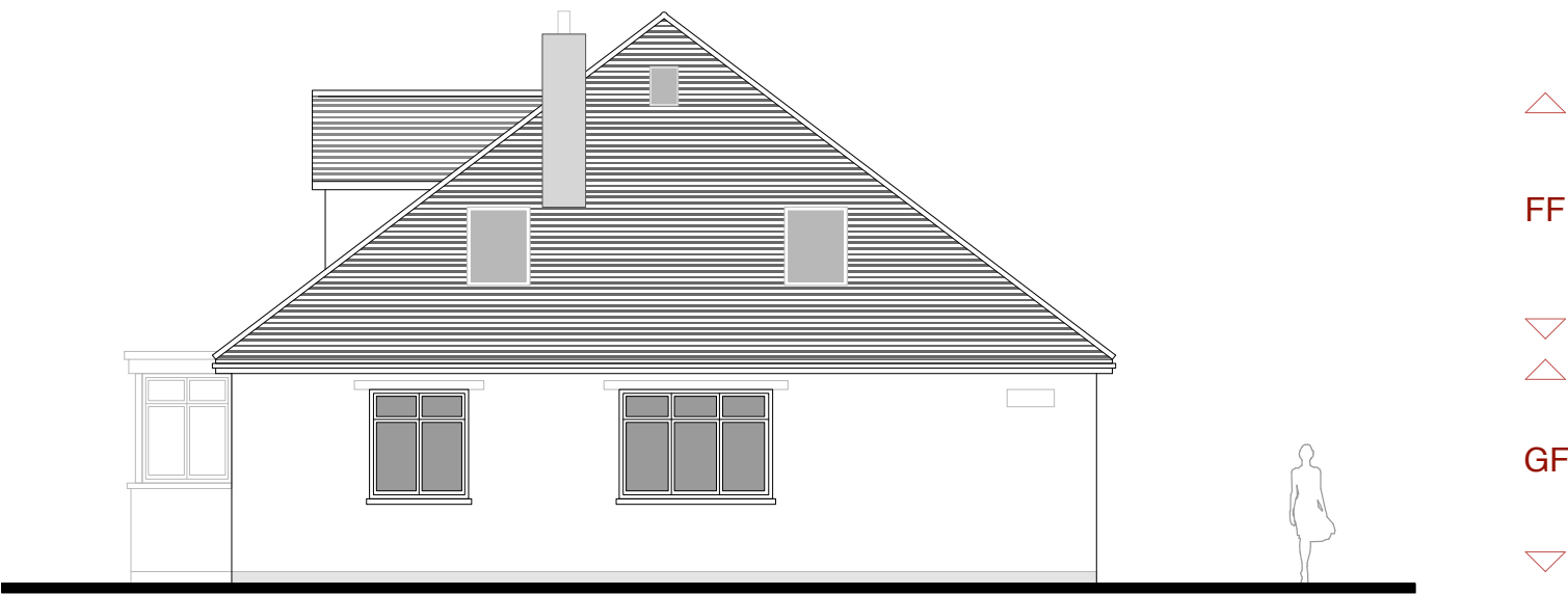
Existing Side Elevation at 1:100 scale
