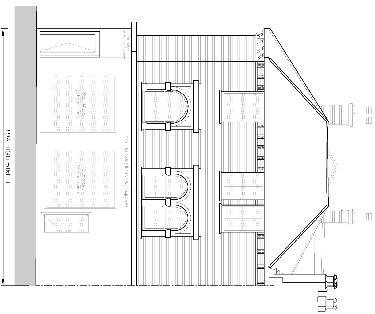
EXISTING HIGH STREET NORTH-WEST ELEVATION. SCALE 1:100.
