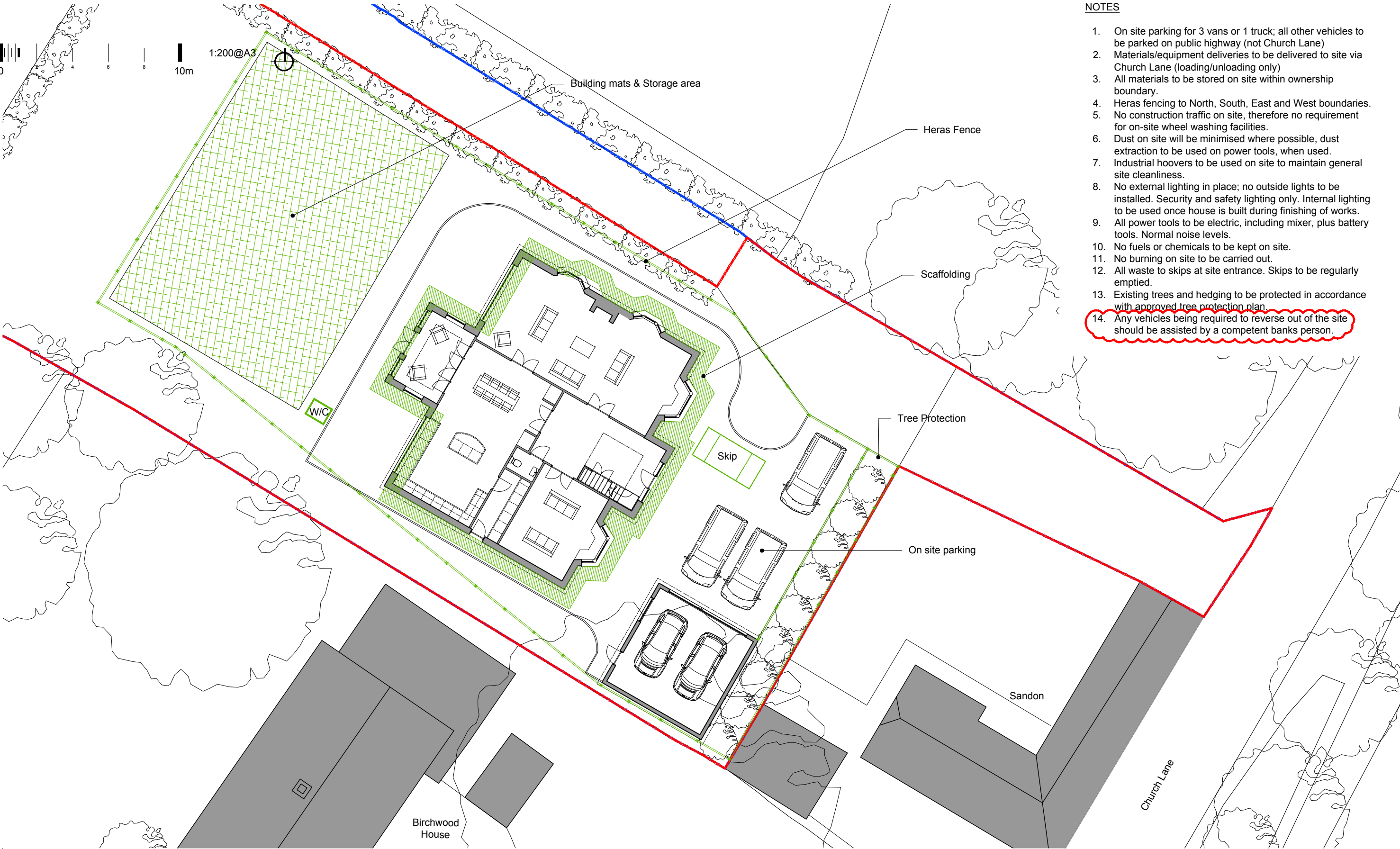
Site Layout Plan - Site set-up during construction
