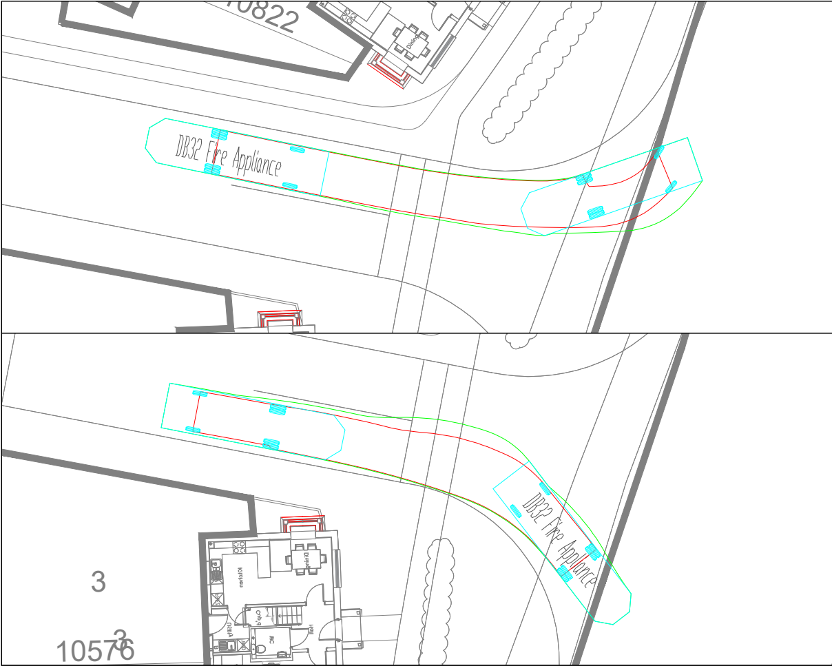
ENTERING AND EXITING THE SITE
