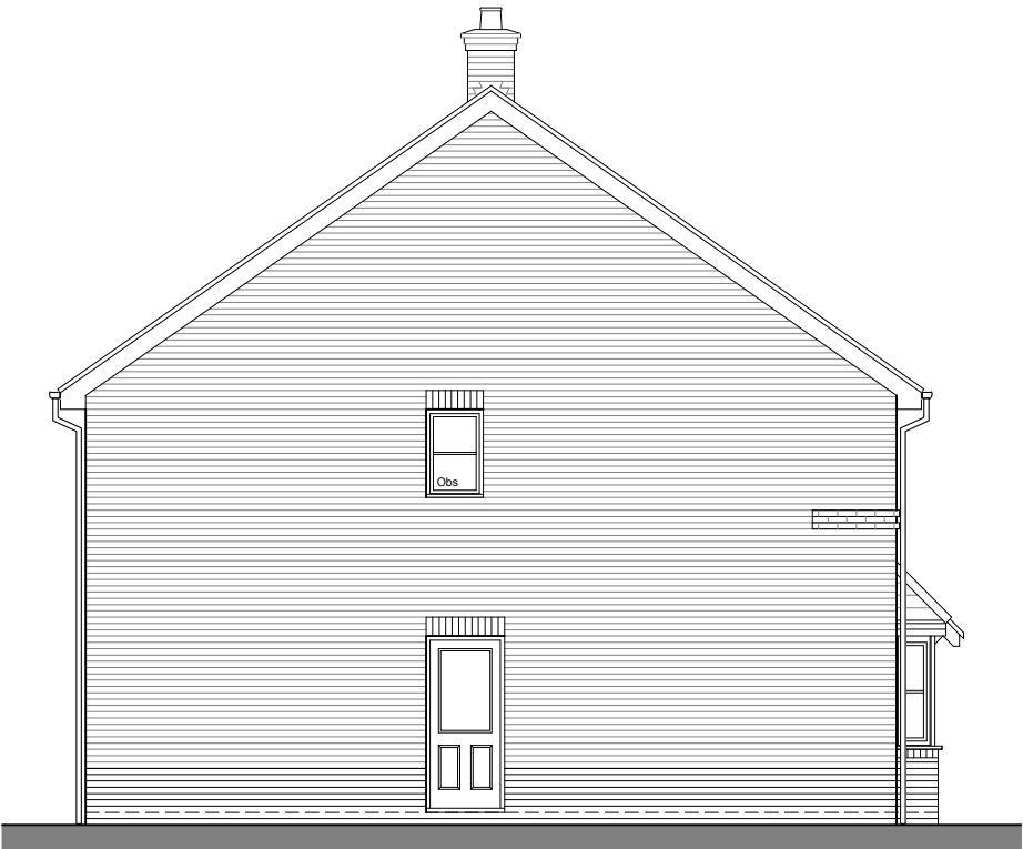
Side Elevation *Obs - Obscured Glass
