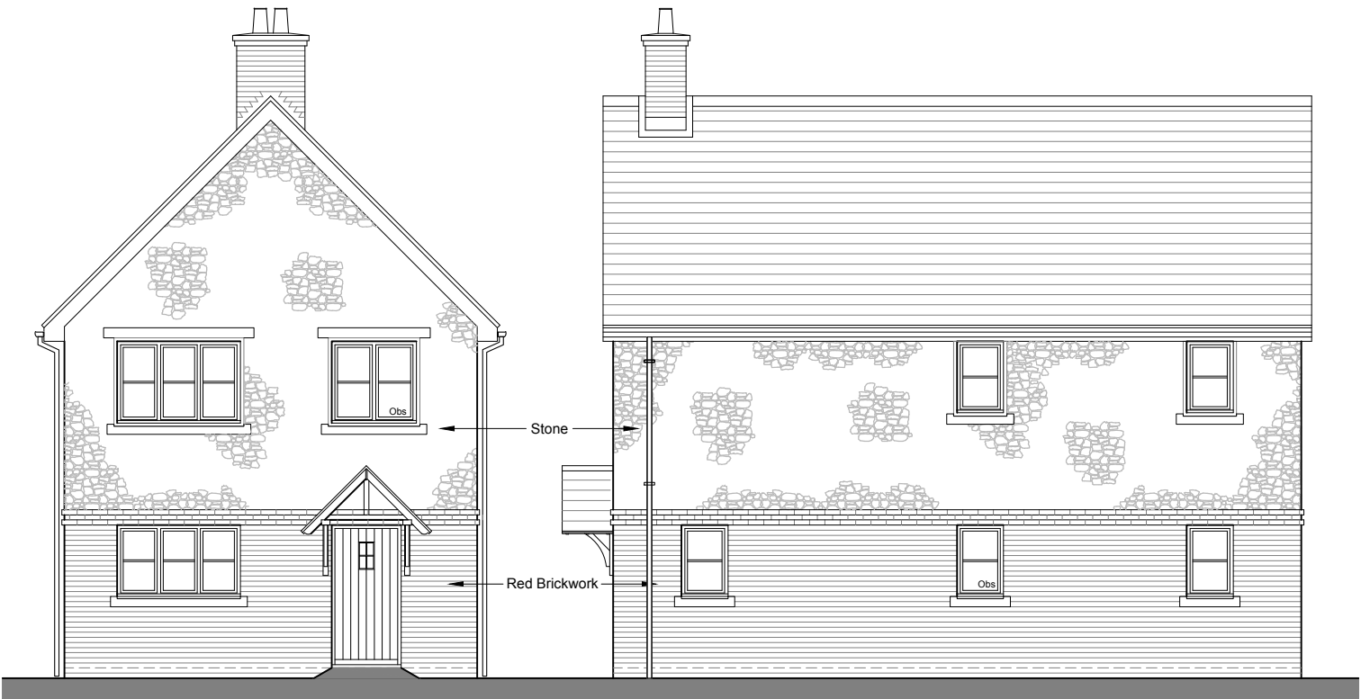
Front Elevation *Obs - Obscured Glass
