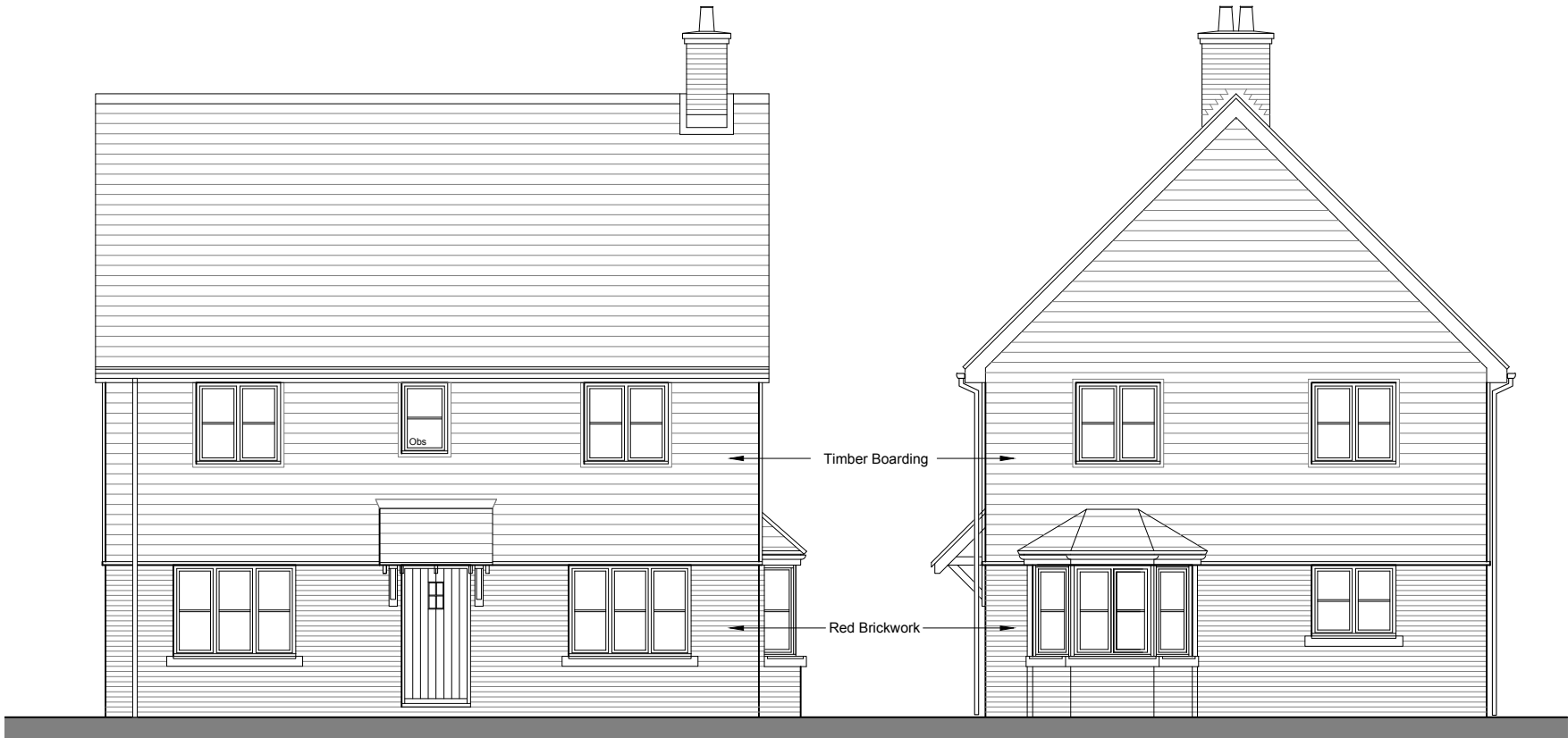
Front Elevation *Obs - Obscured Glass
