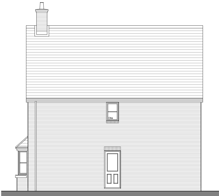
Rear Elevation *Obs - Obscured Glass
